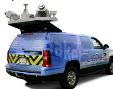
Figure 3.1 Mobile LiDAR Unit
