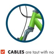
cracks, crimps, rust, or dirt
