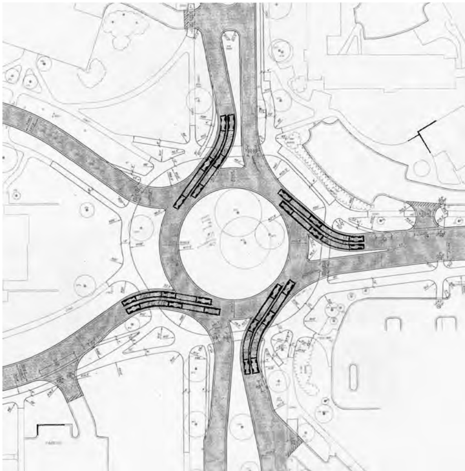
Figure 79. Natural vehicle paths in a multilane roundabout with narrow entry and circulatory roadway widths.
