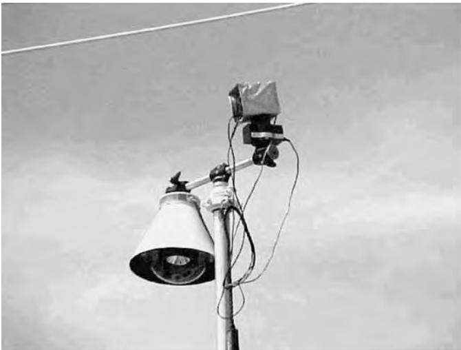
Figure 6. Omnidirectional camera and digital camera located at top of mast.
