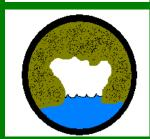
The build-up increases over time when grease and other debris are washed down the drain.
