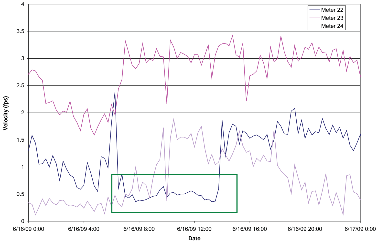
Figure 5-16: Velocity Readings for Meters 22, 23 and 24 During 6/16/2009 Wet Weather Event
