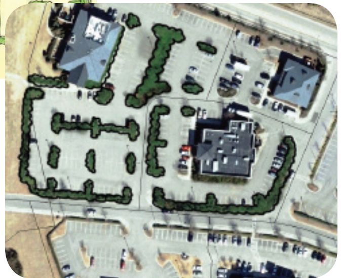
DEFINING PARKING WITH PERIMETER LANDSCAPING AND INTERNAL LANDSCAPING TO DEFINE PARKING PODS
