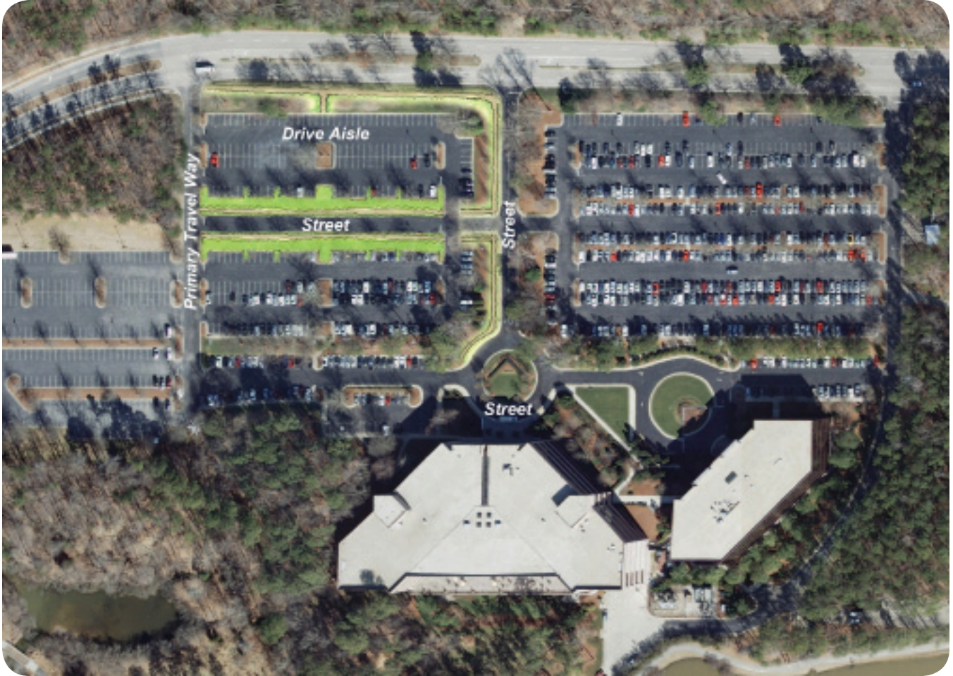
THE PARKING LOT ON THE LEFT HAS BEEN DIVIDED INTO TWO PODS BY ADDING A STREET. THIS ELIMINATES THE "SEA OF PARKING" PERCEPTION.
